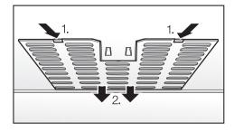
Release the filter cover ①, then lower it together with the filter mat and remove ②.
